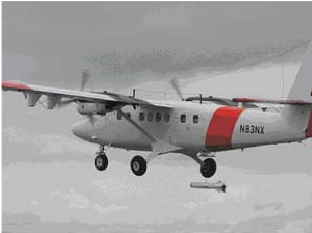
Figure 10. Photo (courtesy Zivko Aeronautics) of the towed vehicle (STV) being lowered from the CIRPAS Twin Otter. In operation it would be up to ~1000 feet below the towing aircraft.
